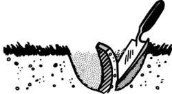
Figure 3. Soil sampling with a trowel.
